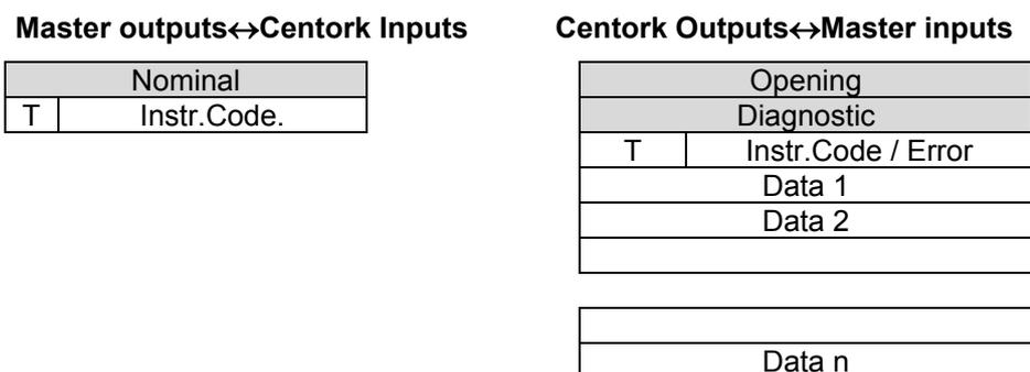
The structure is formed by 22 bytes max. that will be transferred by the PROFIBUS-DP fieldbus.
