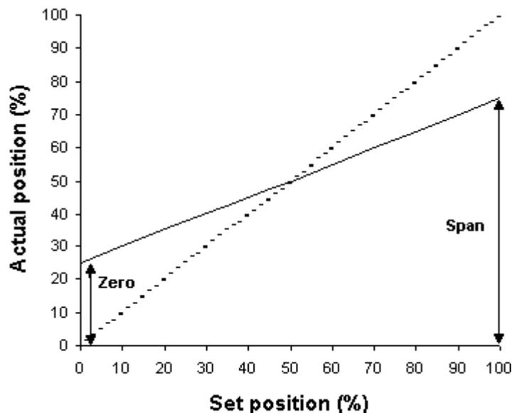
Zero and span for TPS (position transmitter)
